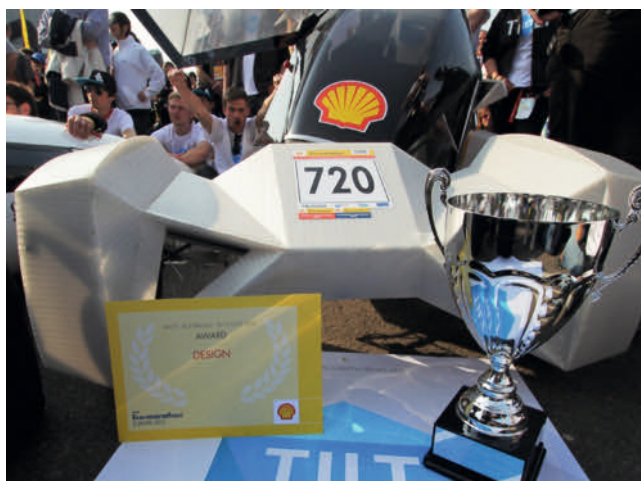
Fig. 6. Vehicle envelope made from lignin-containing ThermHex sandwich panels (photo: Burg Giebichenstein Kunsthochschule Halle)
