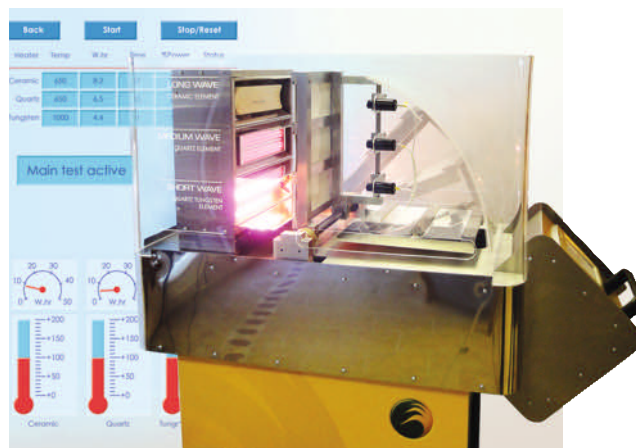
Fig. 4. Testing arrangement for determining the best wavelength for infrared heating (photo: Friedr. Freck)
