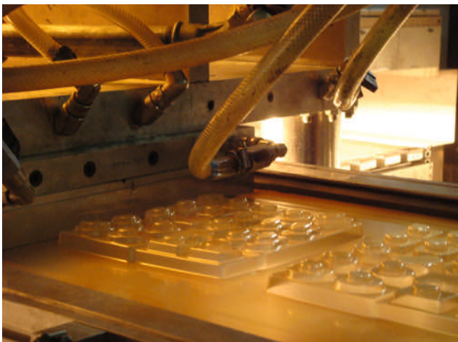
Fig. 3. Thermoforming of corn starch-based film through use of optimized teaching (photo: Heraeus)
