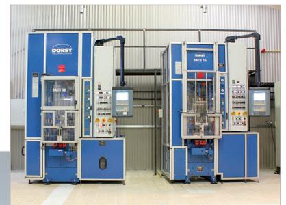
Ceramicx manufactures dust press components on Dorst 20 and 15 tonne presses ( shown above ) and a Dorst 6 tonne press
