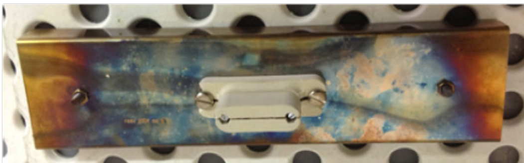
Figure 1: Discoloured stainless steel body,
