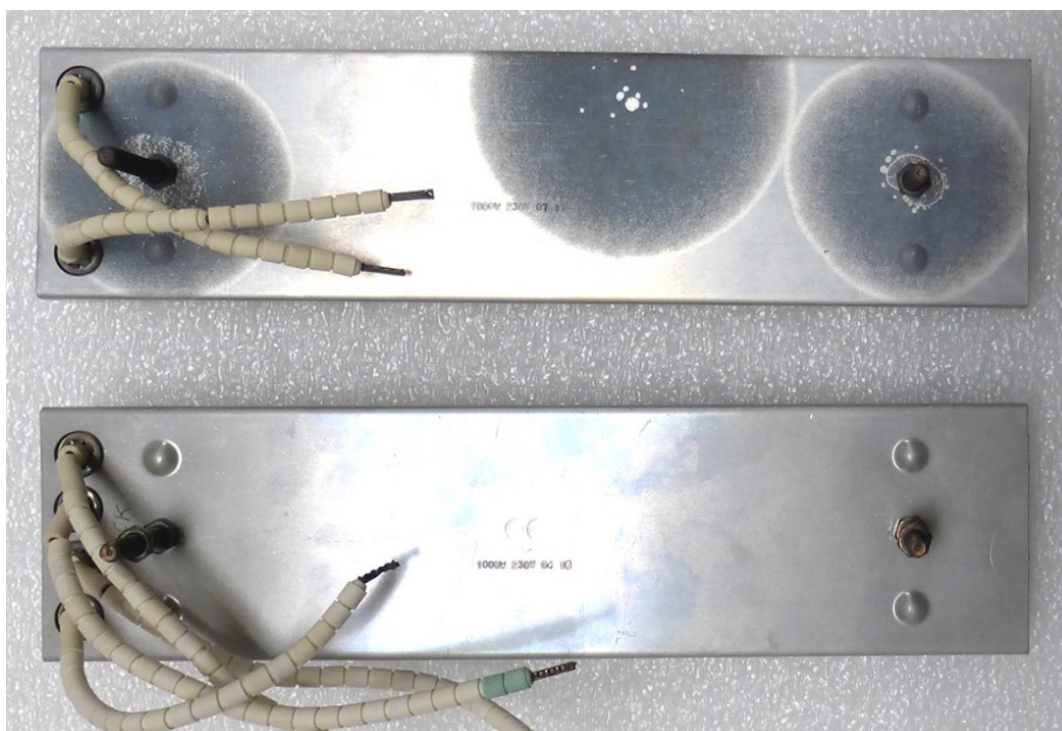
Figure 2: Difference in the back surface of the two FQE bodies (competitor - above, Ceramicx - below) after cooling to room temperature
